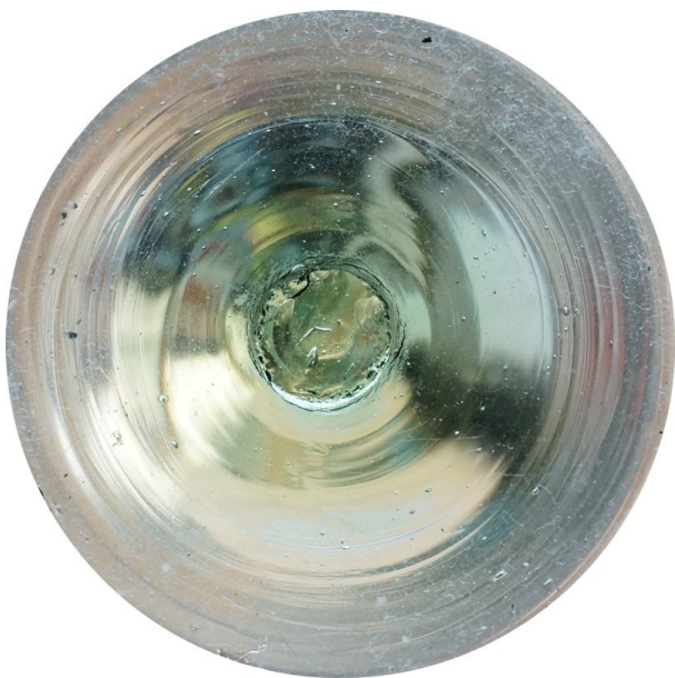
A bull's-eye from a crown glass disc
