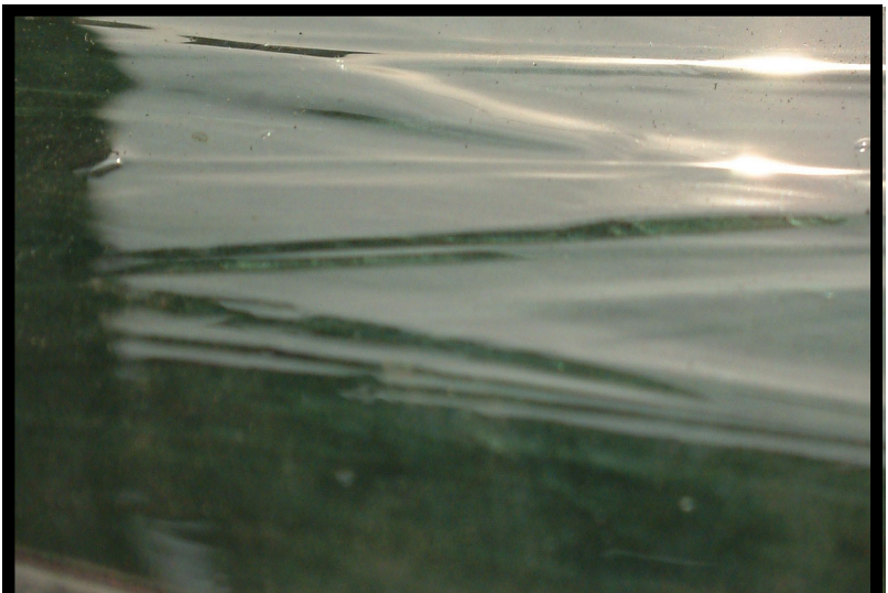
Cylinder glass - rather more uneven but parallel ripples.
