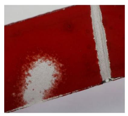
This is a piece of flashed red glass where I have ground a groove and sandblasted a patch of the red layer away. I didn't polish these areas! Top image is of the red side, middle is edge on and bottom is through the clear carrier layer.
