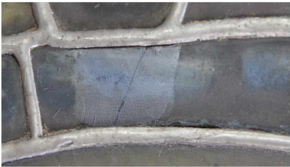
Fracture after polyester has been applied (reflected light)
