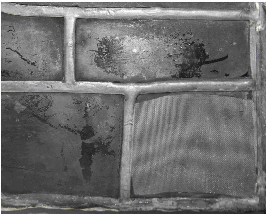
White polyester against clear glass in reflected light (left) and transmitted light (right)
