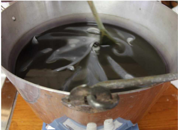
LEFT: STIRRING THE DYE TO ENSURE EVEN COLOUR DISTRIBUTION RIGHT: COLOURED POLYESTER PRODUCED WITH THE DYES
