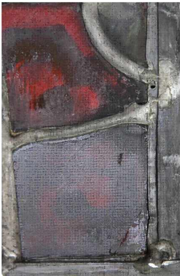
Fracture after polyester has been applied (back reflected light)
