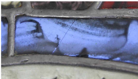
Fracture after polyester has been applied (transmitted light)
