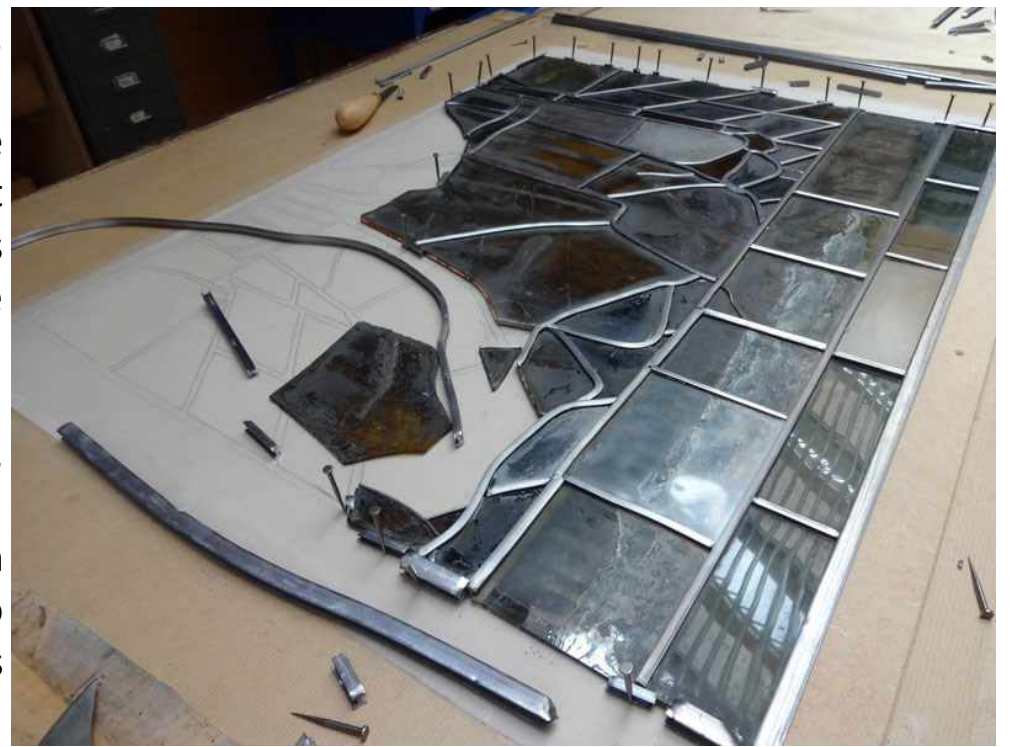
A PANEL DURING ASSEMBLY – NOTE THE DESIGN ATTACHED TO THE BOARD BELOW THE GLASS, AND THE NAILS HOLDING THE PIECES IN PLACE.
